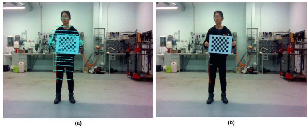
Figure 8. Illustration of the radar-LiDAR-camera. (a) Overposed LiDAR point cluster as extracted using the radar point as a reference, and (b) projection of the radar data onto the camera image.
