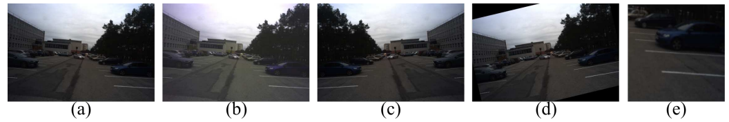
Figure 4. Data augmentation processes: (a) is the original image, (b) is color jitter, (c) is horizontal flip, (d) is random rotate in the range (-20^\circ, 20^\circ) , (e) is the random crop of dimension 128 \times 128 .
